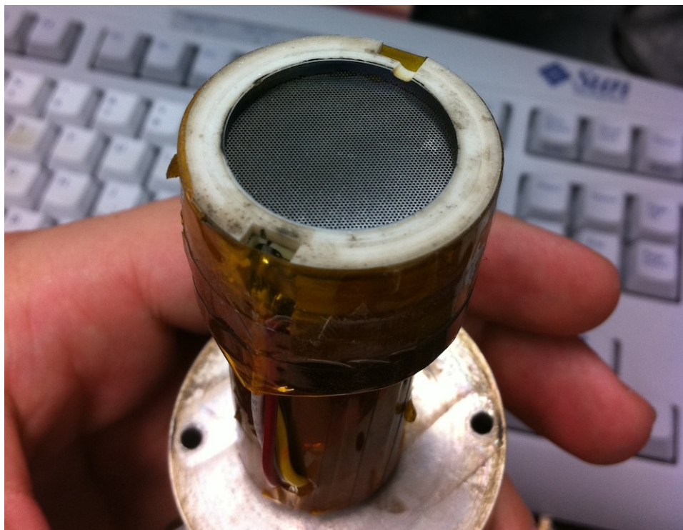
FIGURE 5.6: Four-grid analyzer with cover removed, showing plasma-facing grid.
