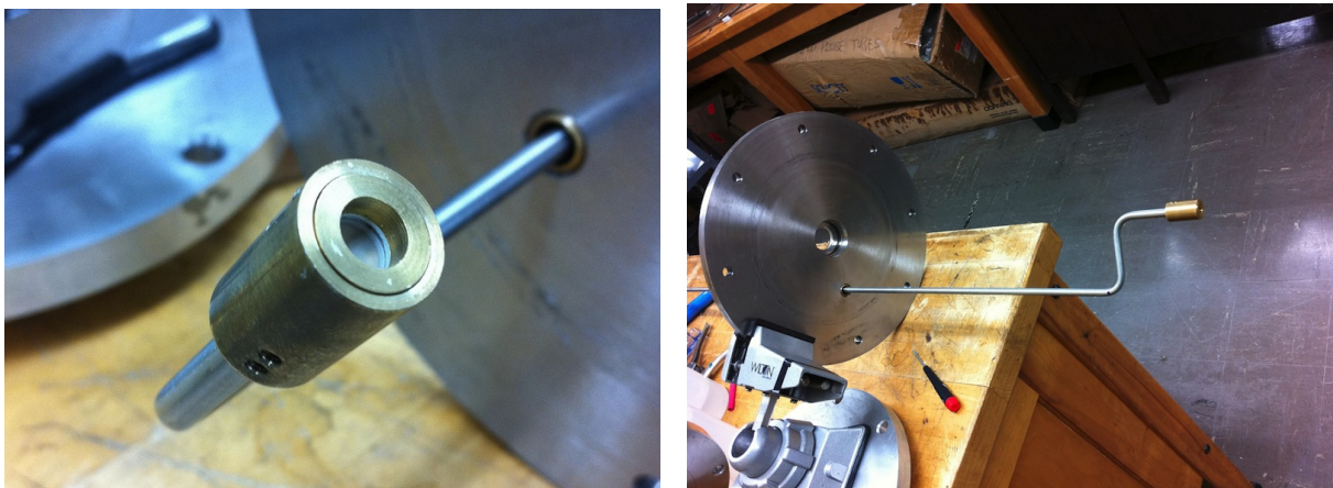
FIGURE 5.3: Two-grid RPA. (a) 2-grid RPA installed on 1/4" stainless shaft, rotated 90° (not facing ion beam) (b) Stainless steel shaft orientation for measurement of beam ('dogleg').
