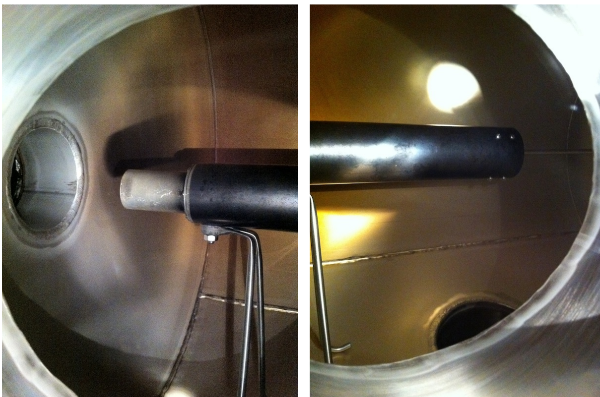
FIGURE 5.8: Four-grid RPA. (a) Front of RPA as installed. (b) Rear of RPA as installed, showing probe feedthrough.
